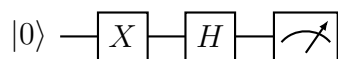
Figure 2.4: A Simple Quantum Circuit Featuring a Pauli-X Gate and a Hadamard Gate
